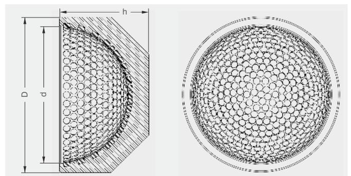
GGB-DB® bearings are made-to-order items. Custom-manufactured to specific requirements, they can readily be produced from drawings providing special dimensions and tolerances, and in forms not included in the following table such as axial and radial segments, half-shells and others. For reasons of economy, however, the types and sizes shown in the following tables should be used whenever possible.
