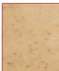
CuSn8 with Composition Sn 8 % P < 0,05 % Cu Rest
