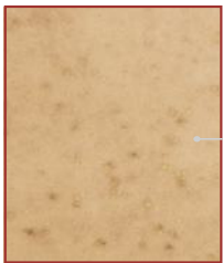
CuSn8 with Composition Sn 8 % P < 0.05 % Cu Rest
